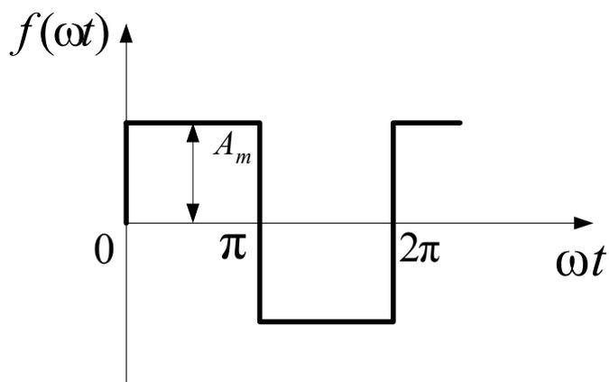
$$f(\omega t) = \frac{4 \cdot A_m}{\pi} \cdot \left( \sin \omega t + \frac{1}{3} \cdot \sin 3\omega t + \frac{1}{5} \cdot \sin 5\omega t + \dots \right)$$
