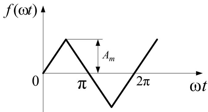
$$f(\omega t) = \frac{8 \cdot A_m}{\pi^2} \left( \sin \omega t - \frac{1}{9} \cdot \sin 3\omega t + \frac{1}{25} \cdot \sin 5\omega t - \dots \right)$$
