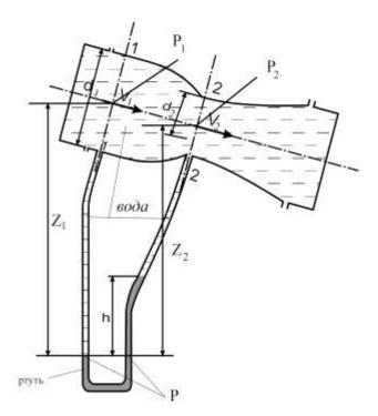
$$z_1 + P_1/\rho g + V_1^2/2g = z_2 + P_2/\rho g + V_2^2/2g + h_{w1-2}z_1$$
